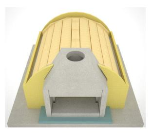
7. Once the first pour of mortar has setup sufficiently hard, place the dome bricks over the jig lengthwise. As always, make adjustments necessary to achieve the best fit and to make sure the nicest side of the bricks are facing down, where they will be seen. Follow these adjustments on every line. Once a good fit has been achieved go to next step.
