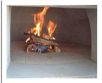
During the second firing, small pieces of firewood are used, to take the oven to higher temperatures than in the first firing. The small fire is kept at the center of the oven floor, and the flames should not reach the top of the dome's interior.
