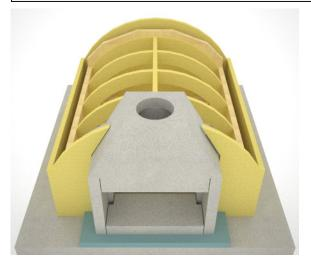
5. Assemble forms using predrilled holes. Place forms flush with front wall. There should be a 1 3/4" gap from the inside of the forms to the side and back wall bricks.
